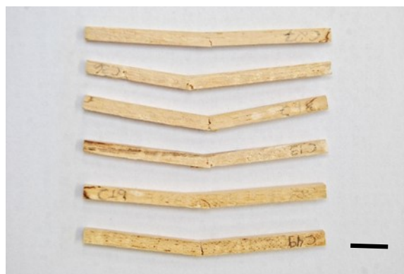
Figure 7. Failure model in the static bending assay: samples from the sibipiruna wood decayed by G. australe , ruptured by simple tension (scale = 1 cm).
