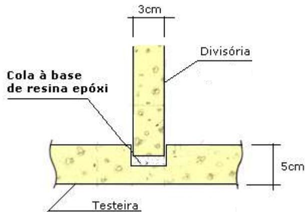
**DETALHE DE ENCAIXE DA TESTEIRA
