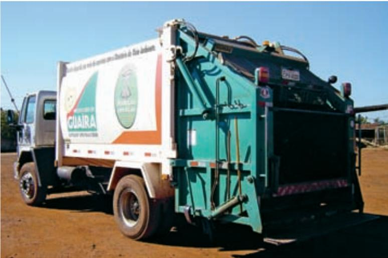
**FIGURA 6** - VEÍCULO PARA COLETA REGULAR, TIPO COMPACTADOR.
